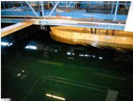
Hull resistance test at model tank
