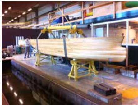
The hull model at towing tank
