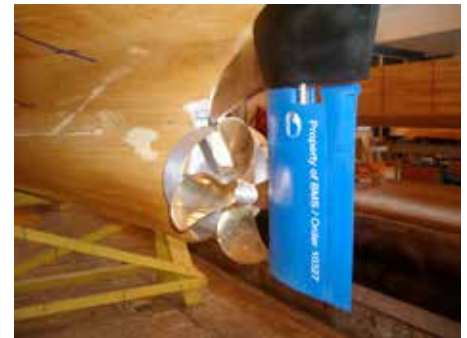
The hull model with design propeller, Mewis duct and Becker flap rudder
